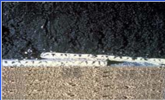
1. Bentonite Installed Dry
