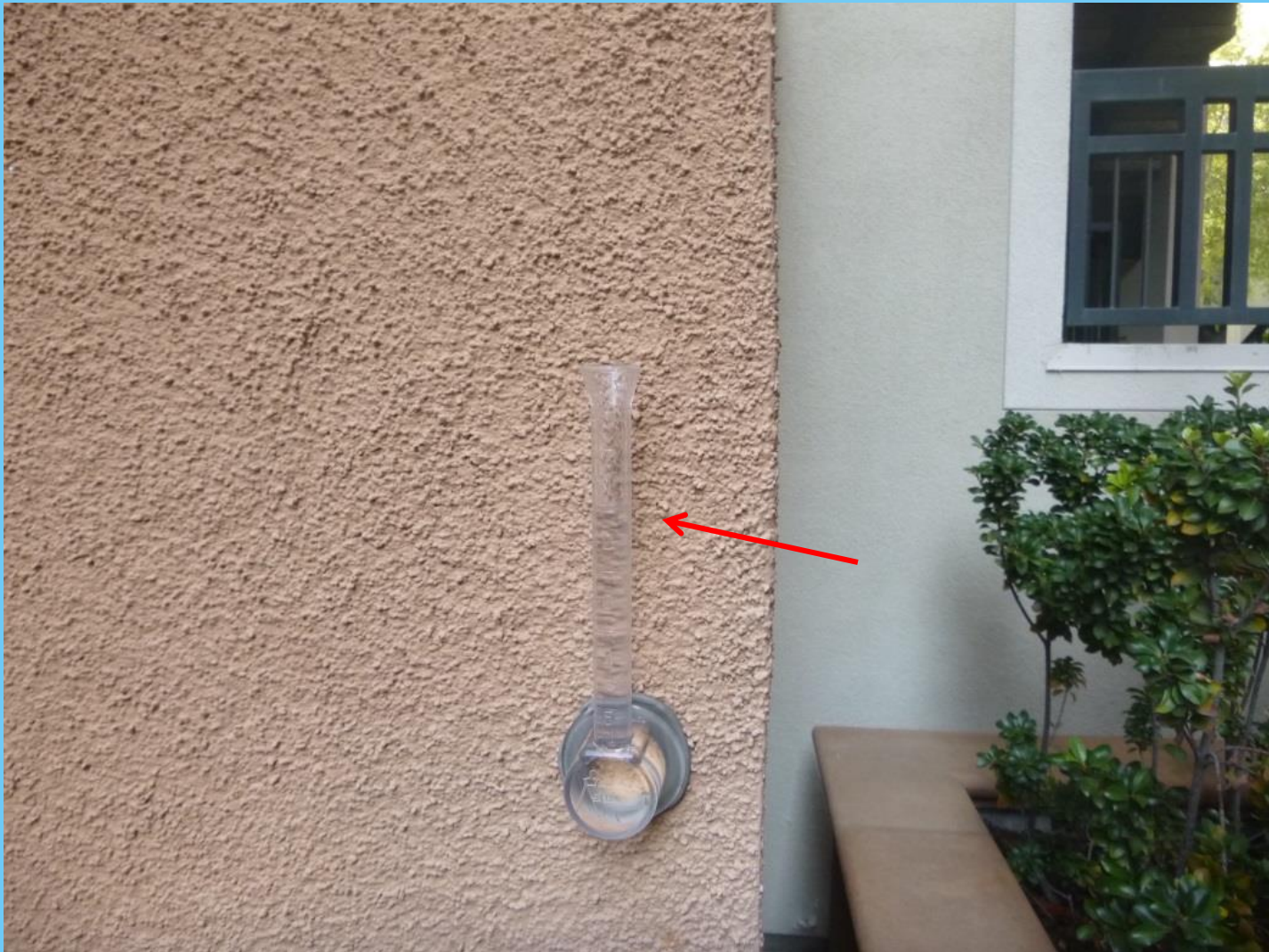
Building 4-Location 8-A. Water dropped to a level almost immediately before we could take a photo of full tube.
