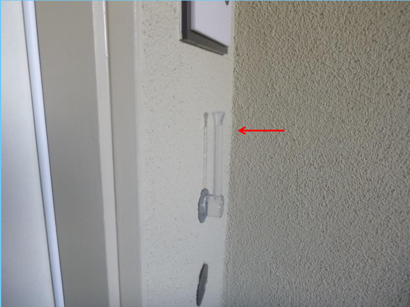
Building Pines B-1 Bldg. 2 Unit 2110 Rilem test over new BMI stucco-tube is full at end of test.
