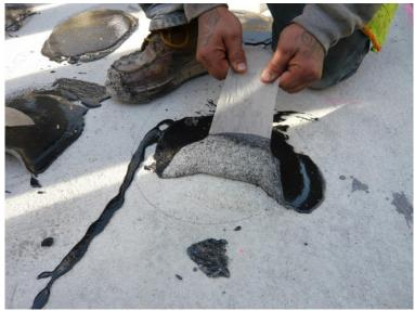
Figure 26: Interestingly, the failure mode is in cohesion of the concrete, as opposed to adhesion of the membrane. The concrete slab surface had improperly cured and was soft and chalky.
