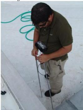
Figure 18: Using potentiometer to discover source of leaks
