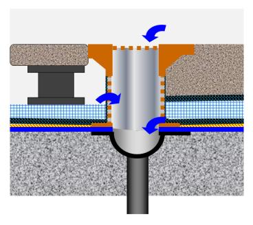
Figure 5: Typical Plaza Drain Configuration
