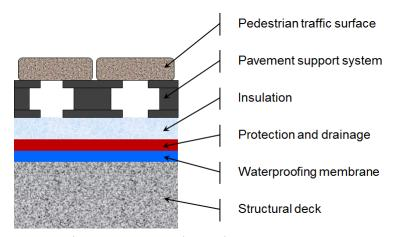
Figure 1: Protected Membrane Components
