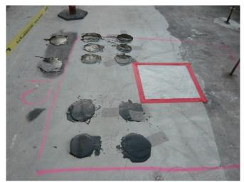
Figure 15: Mat test (Right) and various samples for pull test about to be performed
