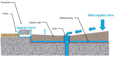
Figure 22: Water flows under the topping slab and appears at door jamb
