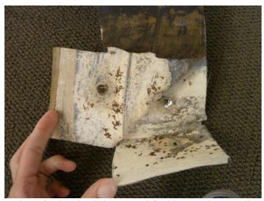
Figure 17: Corrosion of galvanized sheet metal flashings under 90 mils of fluid applied membrane
