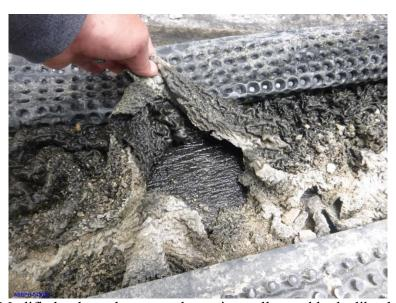
Figure 24: Modified polyurethane membrane is swollen and looks like the texture of "brain" or brainiac. Prolonged immersion of the membrane results in swelling and water absorption far beyond manufacturer's published results.
