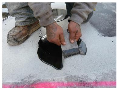
Figure 25: This sample exhibits failure in adhesion due to a water based primer that was used in the application that was not curing due to cold temperature.
