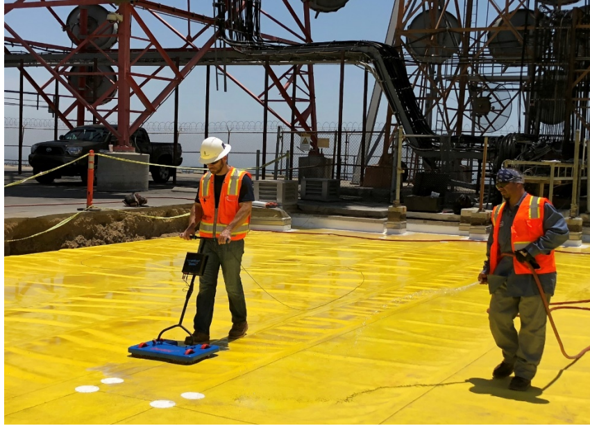
Figure 17 - ELD Low Voltage Horizontal Scanning with Platform
