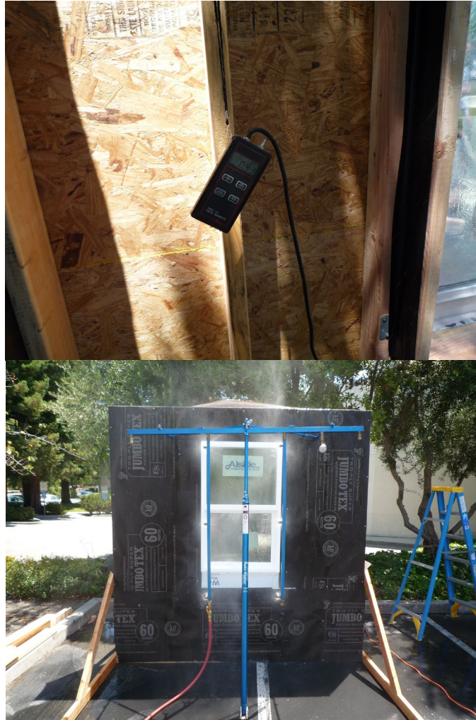
Figure 3 - Mock-Up Testing Of Glazing System with Manometer
