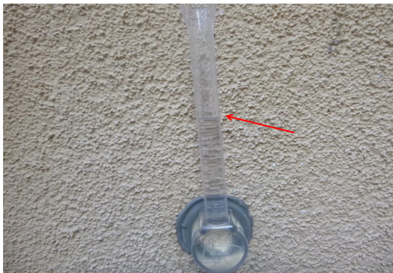
Figure 5: Rilem Tube Level Dropped in 15 Minutes
