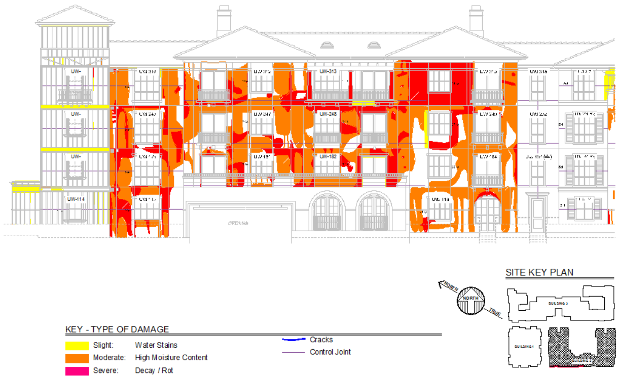
Figure 6A: Damage – South Elevation – Partial
