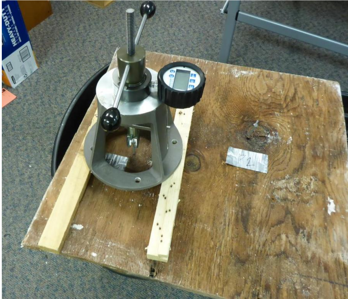
COM-TEN Digital Pull Tester in place during testing
