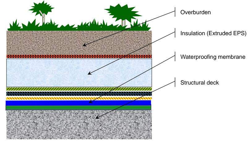
Insulation must have sufficient compressive strength (60 to 100) psi and must not absorb water
