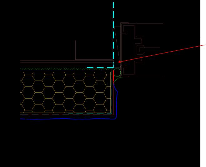
Manufacturer's standard detail is missing secondary seal to water resistive barrier.
