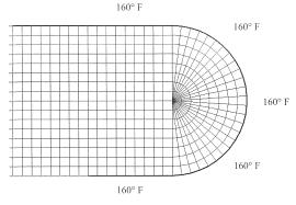
**2D Finite Element Model of EIFS bull-nose Specimen:** Model is subjected to a uniform thermal load of 160 F. Elements are 4 node quadrilaterals and are assigned the
