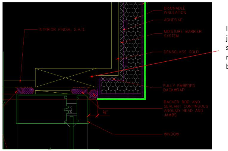
Inside sealant joint to seal secondary moisture barrier.
