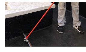
Spark testing is the only ELD test method that does not require water for testing. Spark testing uses high voltage electricity and can effectively test horizontal and vertical areas. This test method may be difficult to test new membranes as they are "sticky" when brooming. Additionally, improper settings of the equipment can damage the membrane. Re-testing after completion of repairs may not be performed immediately.
