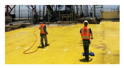
ABB Testing provides specialized Electronic Leak Detection (ELD) and membrane performance testing. ELD is most commonly performed on new membranes for commissioning and integrity testing, but can also be performed on existing construction. ELD detects leaks and voids that other testing equipment cannot locate as accurately.
